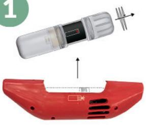
Remove the Pinger from the rubber carrier and unscrew the lid.
