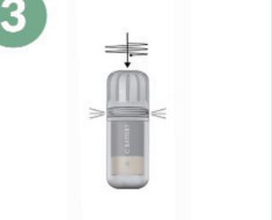
Replace the Pinger lid and tighten down fully, ensuring the O-Ring becomes compressed.
