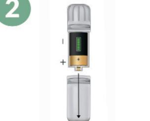
Insert the battery ensuring the polarity is correct.
